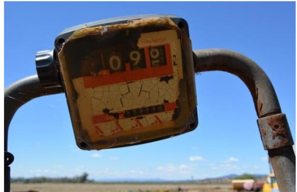
Figure 2: Your records are only as good as your measuring equipment. Faulty gauges and decaying piping and tanks can be a hidden source of fuel wastage (NSW Farmers 2013).
