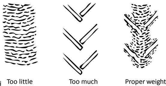
Figure 1: Read your tyre prints. Tread marks provide a rough indicator of correct tyre pressure and tractor set-up. Adapted from (Svejkovsky, 2007).
