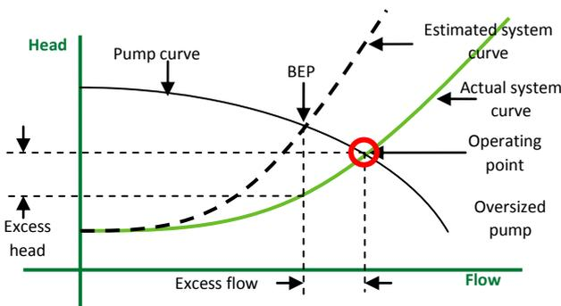
Figure 1: Impact on performance of oversizing pumps.
