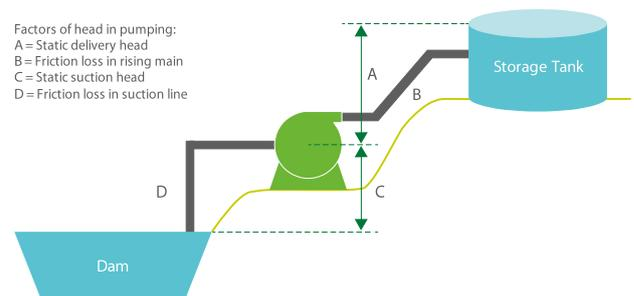
Figure 2: Example of a pump system with a reservoir.
