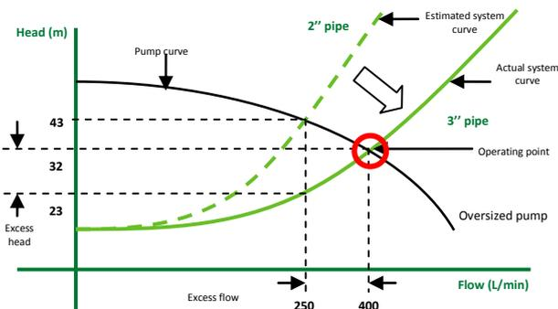
Figure 3: An optimised system, achieved by changing the width of piping from two inches to three inches.
