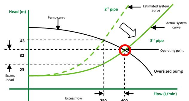
Figure 2: Optimising a system by changing the width of piping from two inches to three inches.
