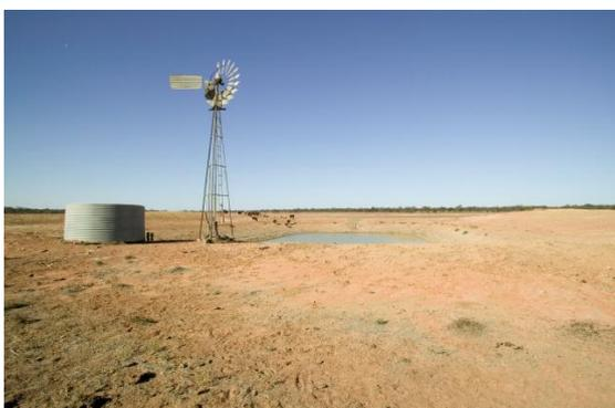
Figure 1: A traditional windmill irrigation set-up, in which wind drives a displacement pump and pulls water to the surface. Although this system uses no energy (other than the wind), it is incapable of moving sufficient amounts of water for most irrigation farms.
