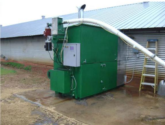
Figure 6: Biomass alternative heating system (University of Georgia, 2009).
