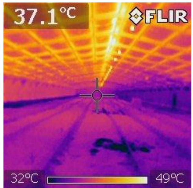
*Figure 1: This infrared photo of a poultry shed demonstrates temperatures within the building. The lights are the hottest items in the shed, at 49 degrees Celsius, while areas of the floor are 32 °C. The air temperature within the shed is approximately 37.1 °C. The shed is in the process of being heated for a new batch of broiler chicks (Image: NSW Farmers 2013, using a FLIR i-7 thermal imaging camera).*
